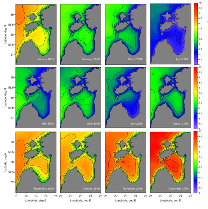
Monthly mean wind speed (m/s) at 10m height in the Gulf of Riga during 2009.
